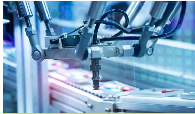
Fixed Flow Controls regulate the action of cylinders in an automated robotic arm.
