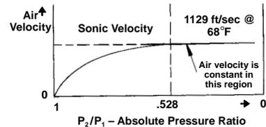
The air flow velocity is limited once the absolute pressure ratio is  $\leq .528$ .
