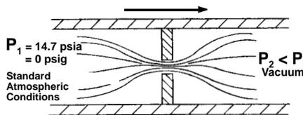
Air at atmospheric pressure enters the orifice and flows to a downstream vacuum pump.
